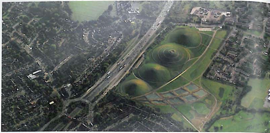
FoRM Associates, Northala Fields (aerial view), 2003–09. Clean demolition spoil, plantings, and water, approximately 2000 x 1500 x 105 ft.
